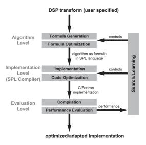
Fig. 1. The program generator SPIRAL
