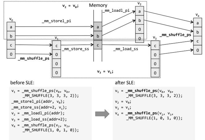
Fig. 5. Example of SLE with load and store intrinsics. Both  $v_0$  and  $v_4$  contain a leftover of length three.
