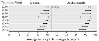
Fig. 10. Each arrow shows an improvement in accuracy of the mvm program. Test (s, p) means an input vector of size  $n = 10^s$ , where p% of the inputs are negative numbers. Arrows start from the accuracy of the interval program without reduction improvement and point to the generated accuracy with reduction improvement.
