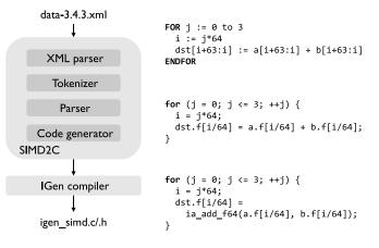
Fig. 4. Generating interval version of SIMD intrinsics from vendor's specification.
