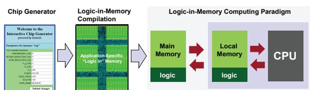
Figure 1: Application-Specific Logic-in-Memory
