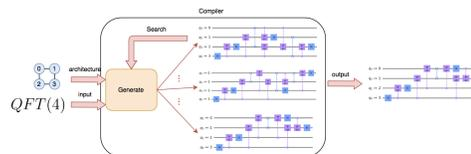
Fig. 1. Proposed generative approach. Example shown is for a 4-qubit quantum Fourier transform (QFT).
