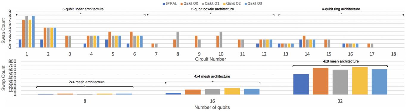
Fig. 2. Swap minimization comparison between SPIRAL and Qiskit on low-level benchmark circuits [top], QFT [bottom]. Target architectures are annotated.
