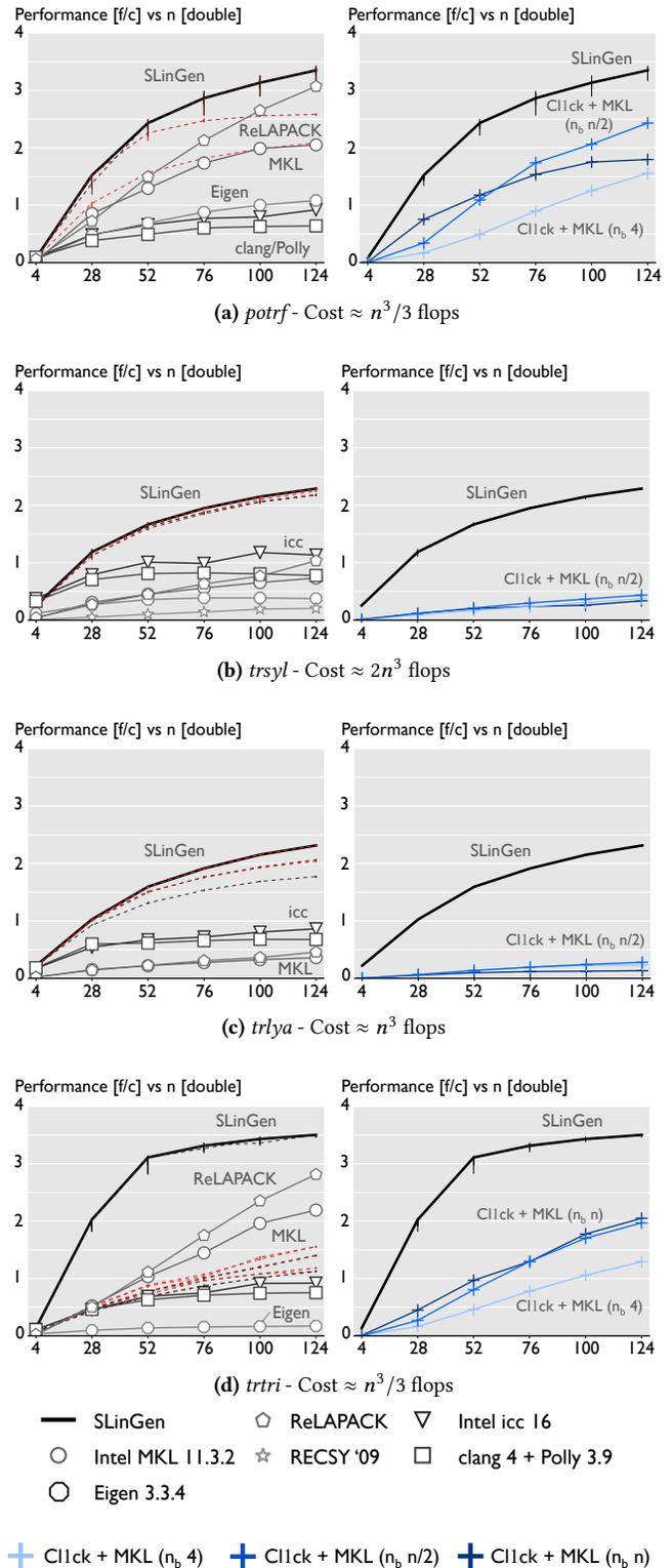
**Figure 14.** Performance plots for the HLAC benchmarks: (a) *potrf*, (b) *trsyl*, (c) *trlya*, and (d) *trtri*. On the left column: colored, dashed lines without markers indicate different `SLiNGEN`-generated algorithms.
