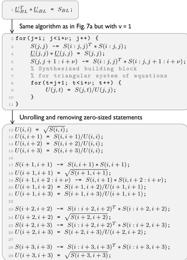
**Figure 9.** Code synthesis for the vector-sized HLAC in line 3 of Fig. 7. We denote with  $i:j$  the interval  $[i, j]$ .
