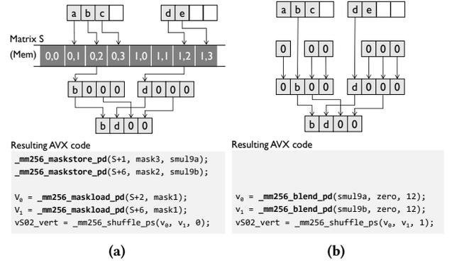
**Figure 12.** Resulting AVX code for the C-IR snippet in Fig. 11 without (a) and with (b) load/store analysis. In (a) `vs02_vert` is obtained by explicitly storing to and loading from memory while in (b) by shuffling vector variables.
