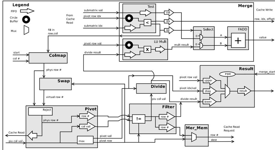
Fig. 2. Pivot and Sub-matrix Update Logic
