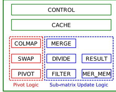
**Fig. 1.** Top Level Sparse LU Hardware Block Diagram
