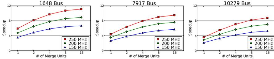
Fig. 5. Performance of Sparse LU Hardware Relative to Benchmark System
