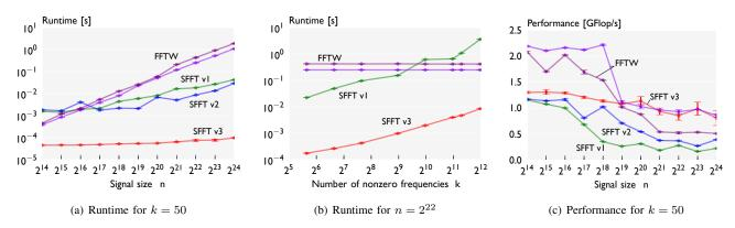
Fig. 2. Runtime and performance benchmarks of our optimized SFFT v1-3 against FFTW. For the performance plots note that the operation counts of the implementations have been reduced compared to the original version.
