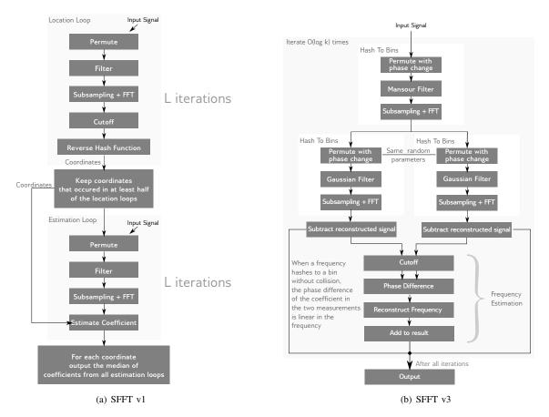
Fig. 1. Algorithm structure of SFFTs
