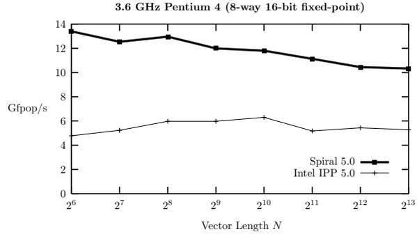
**Figure 2: Vector SIMD. Performance of 1D DFTs, Spiral and Intel IPP 5.0. Higher is better.**
