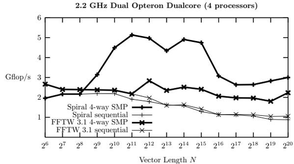
**Figure 3: Multicore CPU. Performance of 1D DFTs, Spiral and FFTW 3.1. Higher is better.**
