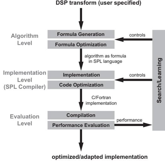
Figure 1: The program generator Spiral.
