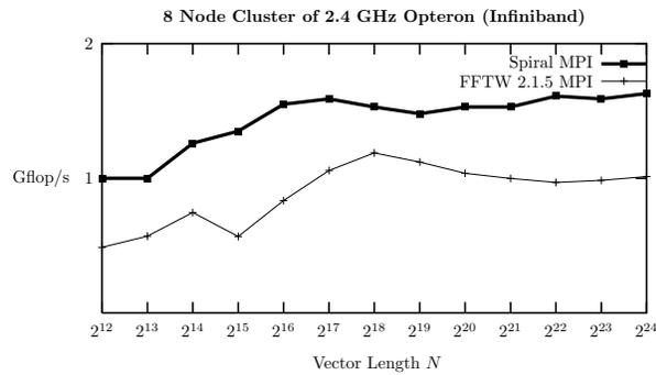
**Figure 4: Message passing. Performance of 1D DFTs, Spiral and FFTW 2.1.5 MPI. Higher is better.**
